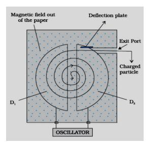
**Construction**: The cyclotron is made up of two hollow semi-circular disc like metal containers,  $D_1$  and  $D_2$ , called dees.
